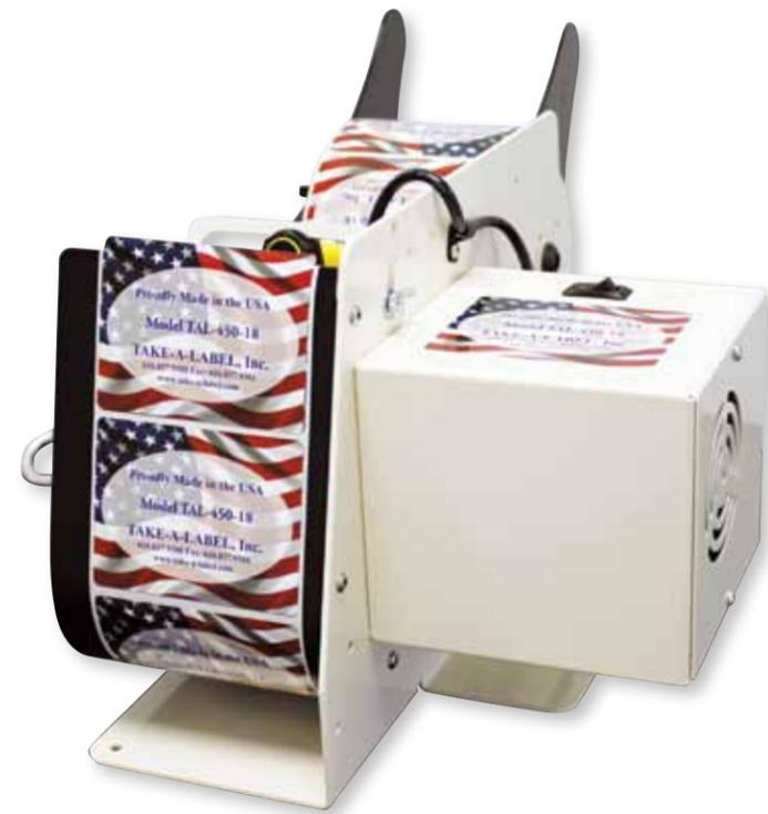
9. Turn on On-Off switch. The waste wind shaft will turn, winding up backing paper and dispensing a label at the top of the peel plate. When the Photo Eye or Micro Switch senses the dispensed portion of the label, the motor will stop. As each label is removed, the machine will operate until the next label is in position to be removed. **(CAUTION:)** Turn off switch before removing wound up waste.
